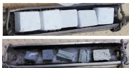
Fig. 2 Appearance of thermal insulations before (upper) and after (lower) reaction test with Cs
