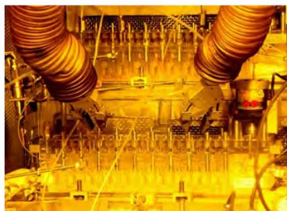
Fig. 2 Mixer-settler extractors and manipulators used in the demonstration test
