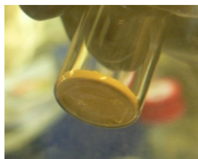
Fig. 2 Precipitation of americium oxalate
