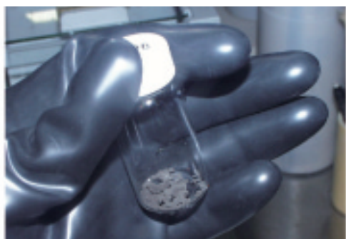
Fig.7-11 PuN powder obtained by nitridation - distillation combined reaction Experiments are carried out in Ar-atmosphere gloveboxes.
