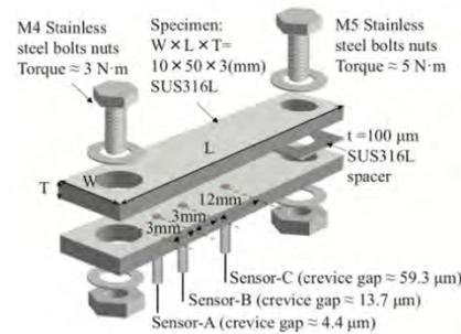
Fig. 2 Schematic illustration of crevice specimen with sensors.
