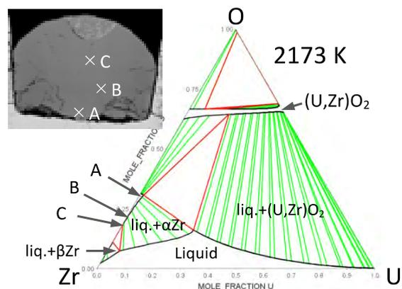
Fig.2 Cross section of test piece and ternary phase diagram of U-Zr-O system at 2173 K.
