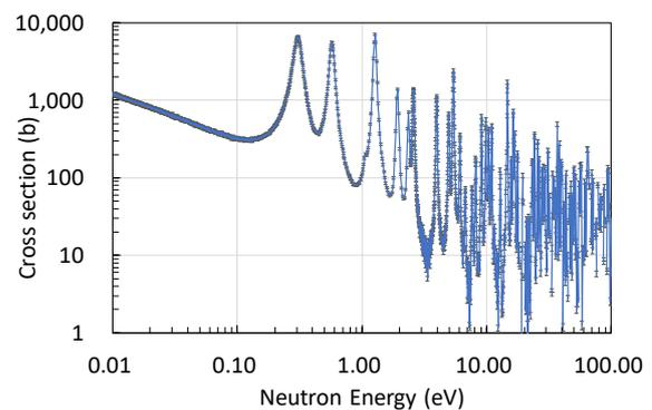
Fig.1 Am-241 neutron capture cross section
