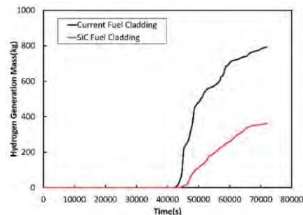
Fig.2 Hydrogen generation mass for current fuel cladding and SiC fuel cladding<sup>2</sup>
