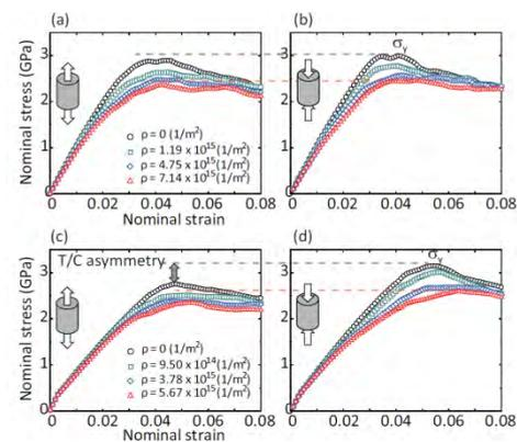
Fig.2 Stress-strain curves and T-C asymmetry in UFG metals: (a) Cu under tension, (b) Cu under compression, (c) Al under tension, and (d) Al under compression.
