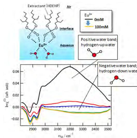
Fig.2 Vibrational spectra of the interface obtained by advanced laser spectroscopy: heterodyne-detected vibrational sum frequency generation spectroscopy
