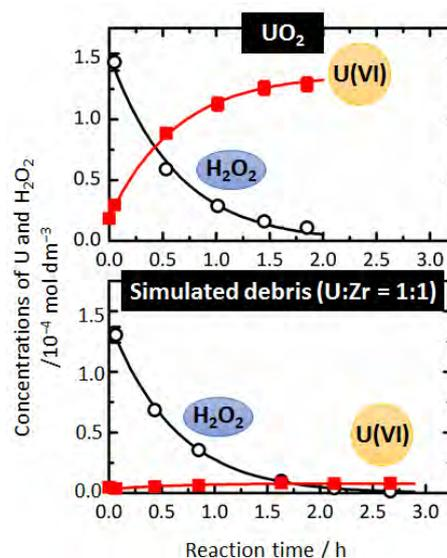
Fig.1 Comparison of the  $\text{H}_2\text{O}_2$  reaction kinetics between  $\text{UO}_2$  and the simulated fuel debris
