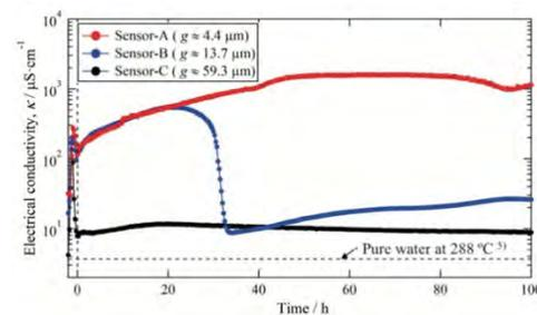
Fig. 3 Change in  $\kappa$  as a function of time in 288 °C pure water with 32 ppm concentration on dissolved oxygen.<sup>2)</sup>
