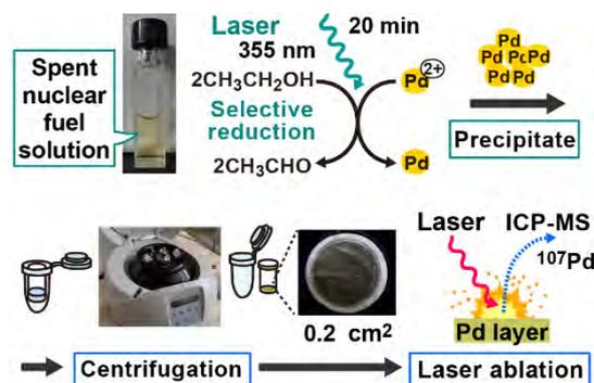
Fig. 2 Direct measurement of  $^{107}\text{Pd}$  by LA-ICP-MS
