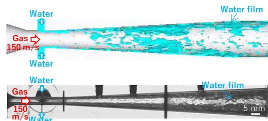
Fig.2 TWO-PHASE FLOW BEHAVIOR IN VENTURI SCRUBBER
