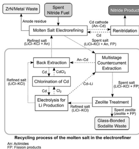
Fig.1 A detailed flowsheet for the electrorefining process.
