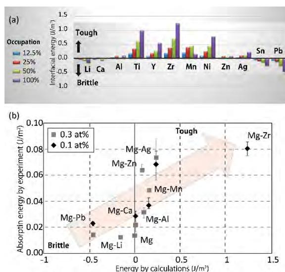
Fig. 2 (a) Energy of interfacial separation in terms of the site occupation. (b) Relationships between experiments and calculations.
