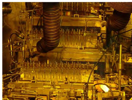
Fig.2 Mixer-settler extractors used in the continuous counter-current experiment to recover Am, Cm, and rare earths by TDdDGA.
