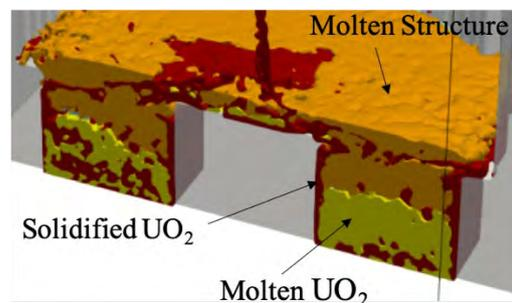
**Fig.1 Interior distribution of accumulated debris (numerical result)**
