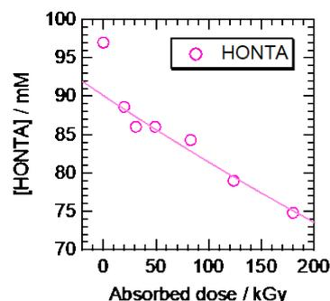
Fig.1 Effects of absorbed dose on concentration of HONTA.
