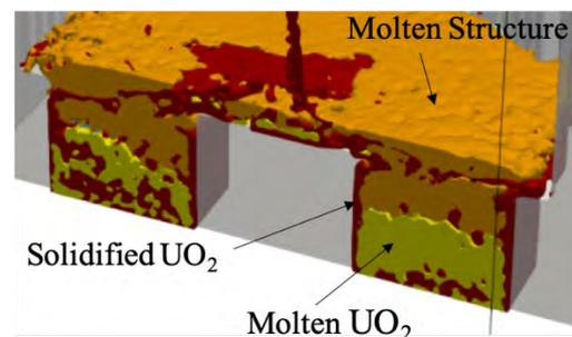
**Fig.1 Interior distribution of accumulated debris (numerical result)**
