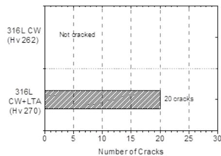
Fig.1 Number of surface cracks in Type 316L SS initiated during CBB testing.
