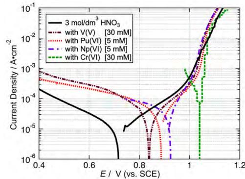
Fig. 1 Polarization curves of SS (SUS310Nb) in the boiling 3 M-HNO<sub>3</sub> containing oxidizing cations<sup>1)</sup>.
