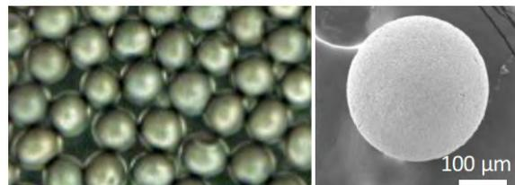
Fig.1  $\text{Dy}_2\text{O}_3+\text{C}$  mixed particles ( $\phi$  0.33 mm) calcined from the gel particles ( $\phi$  0.47 mm).
