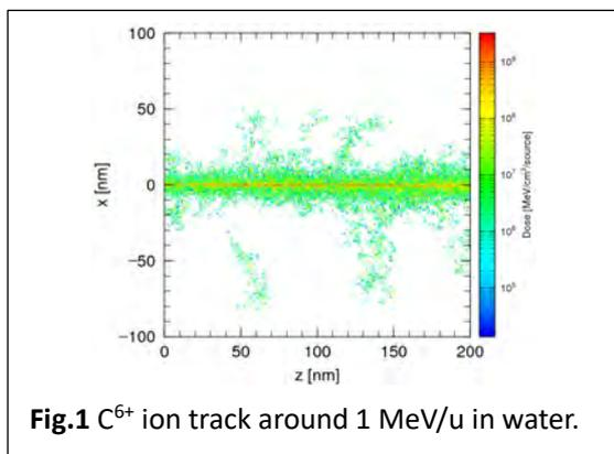
Fig.1  $C^{6+}$  ion track around 1 MeV/u in water.
