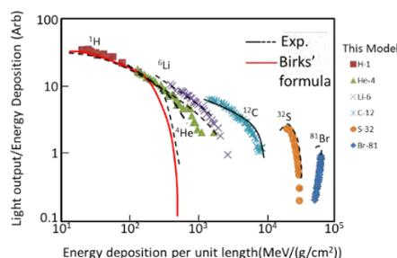
Fig.2 Comparison of scintillation light yield owing to heavy ions
