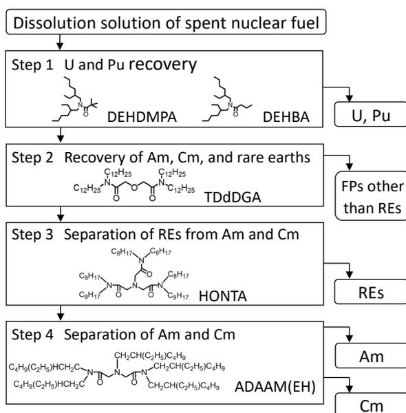
Fig.1 A conceptual flow sheet of SELECT process and proposed extractants in each step
