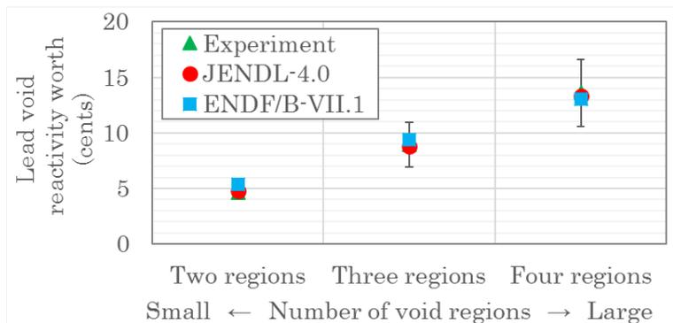
Fig.2 Comparison of experimental and calculated lead-void-reactivity worth in the LEU/Pb systems
