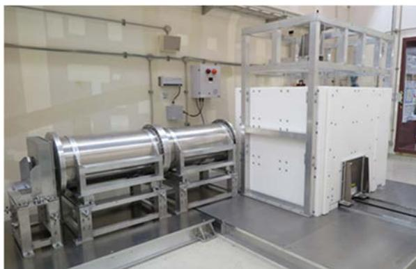
**Fig.1 Active neutron non-destructive analysis system: Active-N**
